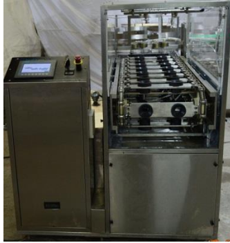
Linear Washer with robotic arms
